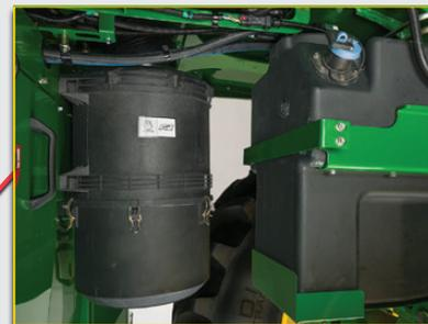
C. Clean diesel exhaust fluid (DEF) tank and pump.
