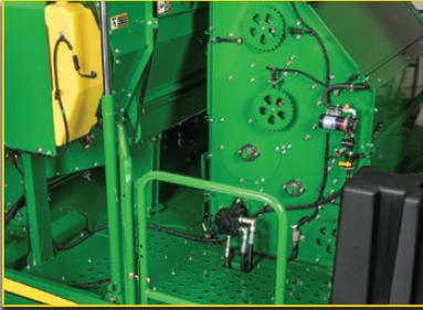
B. Clean behind cab, tanks, ducts, and front of accumulator. Clean and inspect cleaner.
