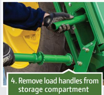
4. Remove load handles from storage compartment
