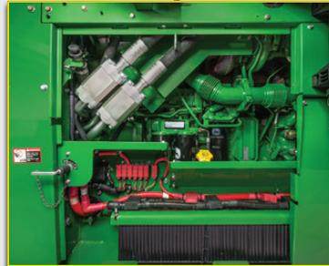
**D.** Clean battery area, rear of engine, exhaust manifold, and turbo.
