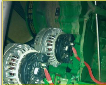
**C.** Clean alternators and check engine belts and pulleys.
