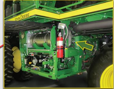
**E.** Thoroughly clean around hydraulic pumps and exhaust components including turbochargers, bellows, and after-treatment devices.
