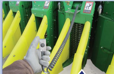
1. Check pressure plate clearance by rotating units slowly using the remote tether switch.
