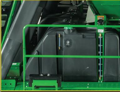
B. Clean behind cab, tanks, ducts, and front of accumulator.
