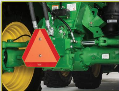
B. Clean rear axle joints, motor, and hoses.
