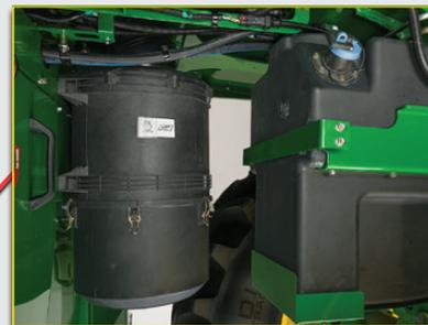
C. Clean diesel exhaust fluid (DEF) tank and pump (if equipped).
