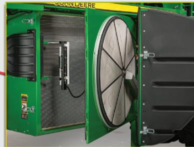
D. Clean cooling module. Open doors to access cooling cores.
